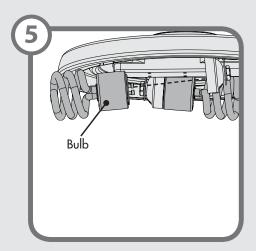
Install a light bulb in each socket.
